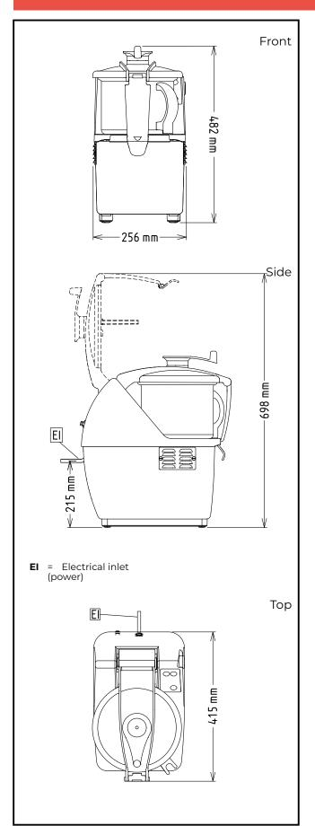
Electric Supply voltage: 600450 (DK55YVV) 200-240 V/1N ph/50/60 Hz Electrical power max.: 1.3 kW **Total Watts:** 1.3 kW Capacity: Performance (up to): 2.5 kg/Cycle Capacity: 5.5 litres Key Information: External dimensions, 256 mm Width: External dimensions, Depth: 415 mm External dimensions, Height: 482 mm
